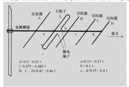
Also can use insulators metal bar! Diagram for wavelength lambda, director, reflector are calculated respectively and the main oscillator length and a, b, c, d spacing after assembled.
