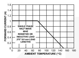
**Figure 1. Forward Current Derating Curve**
